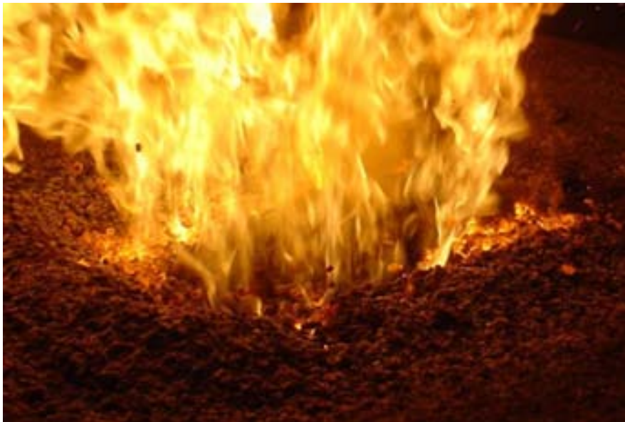
Fig.4: Poor combustion with standard coal grate. Volcano effect with high-temperature, small combustion zones, and airborne pellets.
