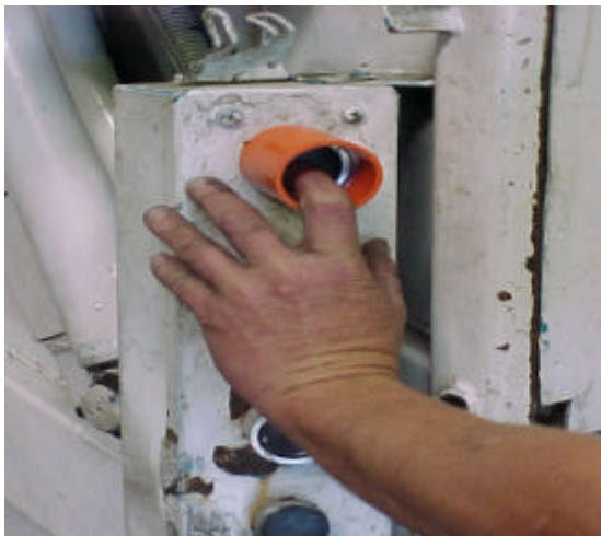
Figure 3: Sheathing of control buttons
