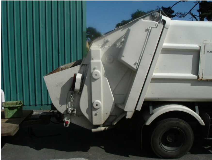
Figure 1: Starting the rear-loading compaction truck
