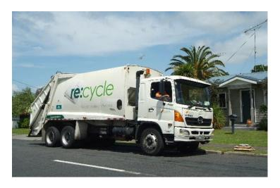
**Figure 12:**One of several types of rear loading collection vehicle in operation in New Zealand
