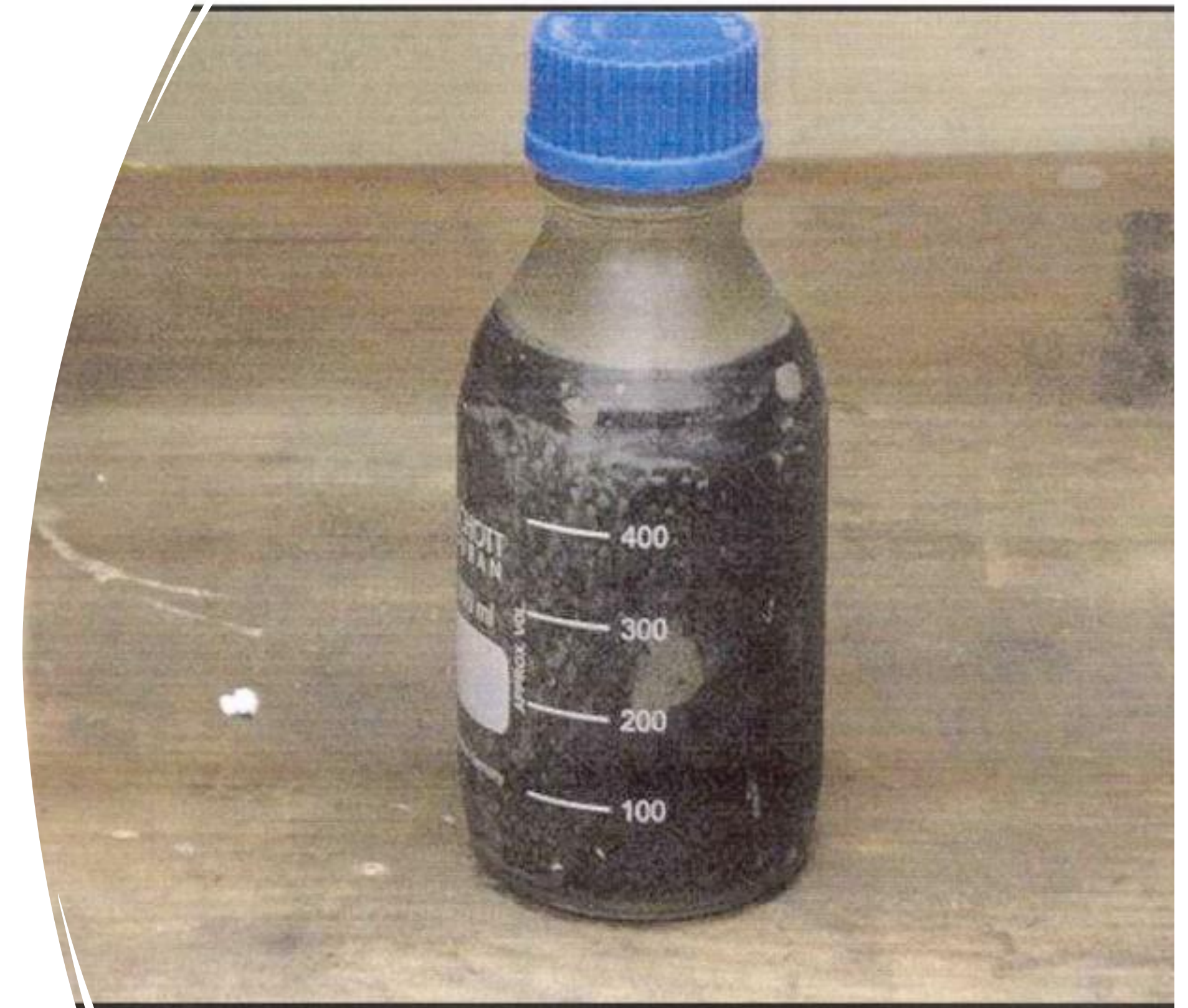
Graph 3: DNAPL product sample. Lighter aqueous phase has suspended sediment resulting in a milky texture.
