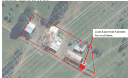
Figure 2 Class B Licensed Asbestos Removal Extent
