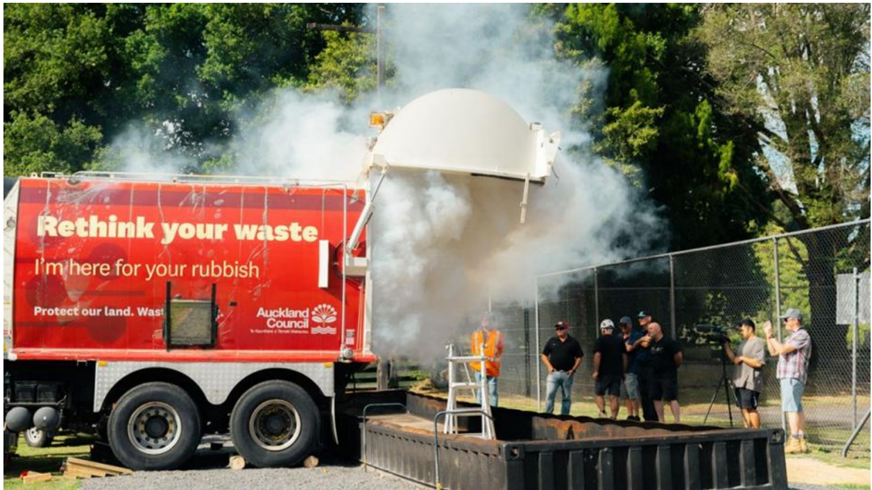
Figure 1-2: Trial Simulation of a Rubbish Truck Li-ion Battery Fire 10
