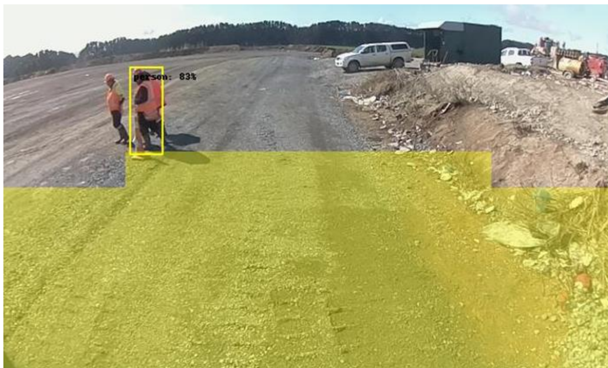
Photo: What an operator would see from the VDU. This shows a person in the 'alert' zone (shaded yellow), detected with 83% confidence.
