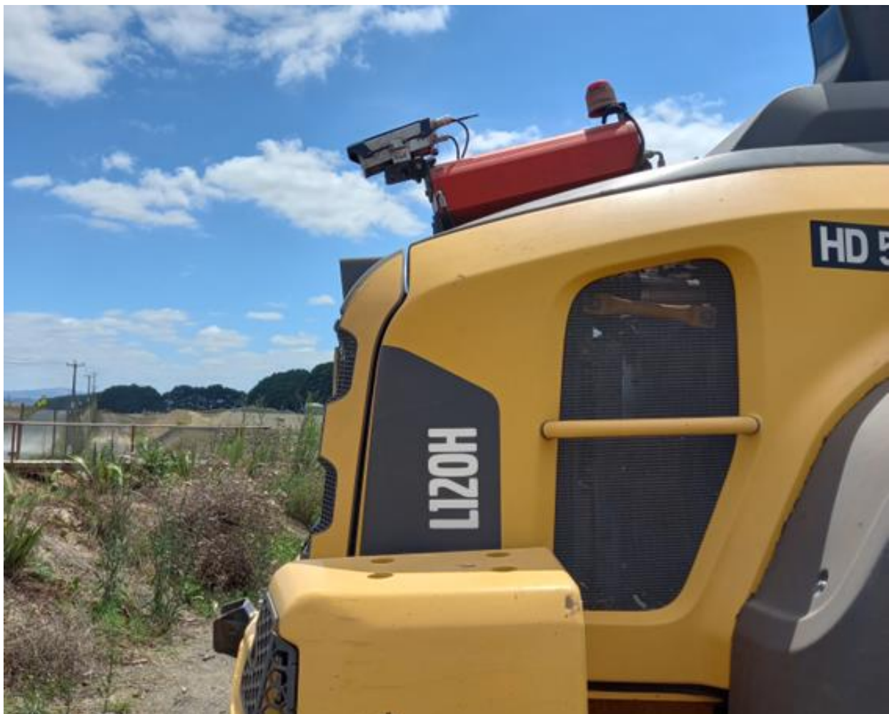
Photo: The camera installed on the rear of a Volvo L120 loader at Hampton Downs Landfill.
