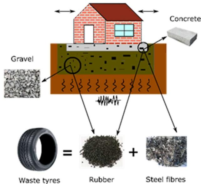
**Figure 1. Eco-rubber seismic isolation foundation system.**
