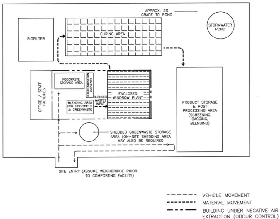
**Figure 2: Enclosed Windrow Composting Facility Layout Schematic (not to scale)**
