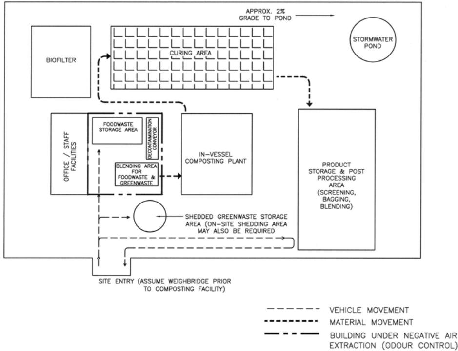
**Figure 1: In-vessel Composting Facility Layout Schematic (not to scale)**
