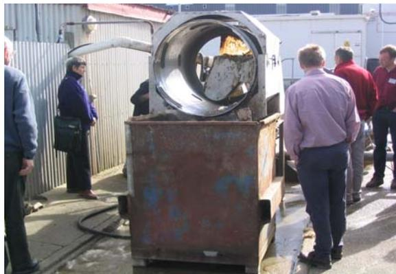
Figure 7: Waste solids separation
