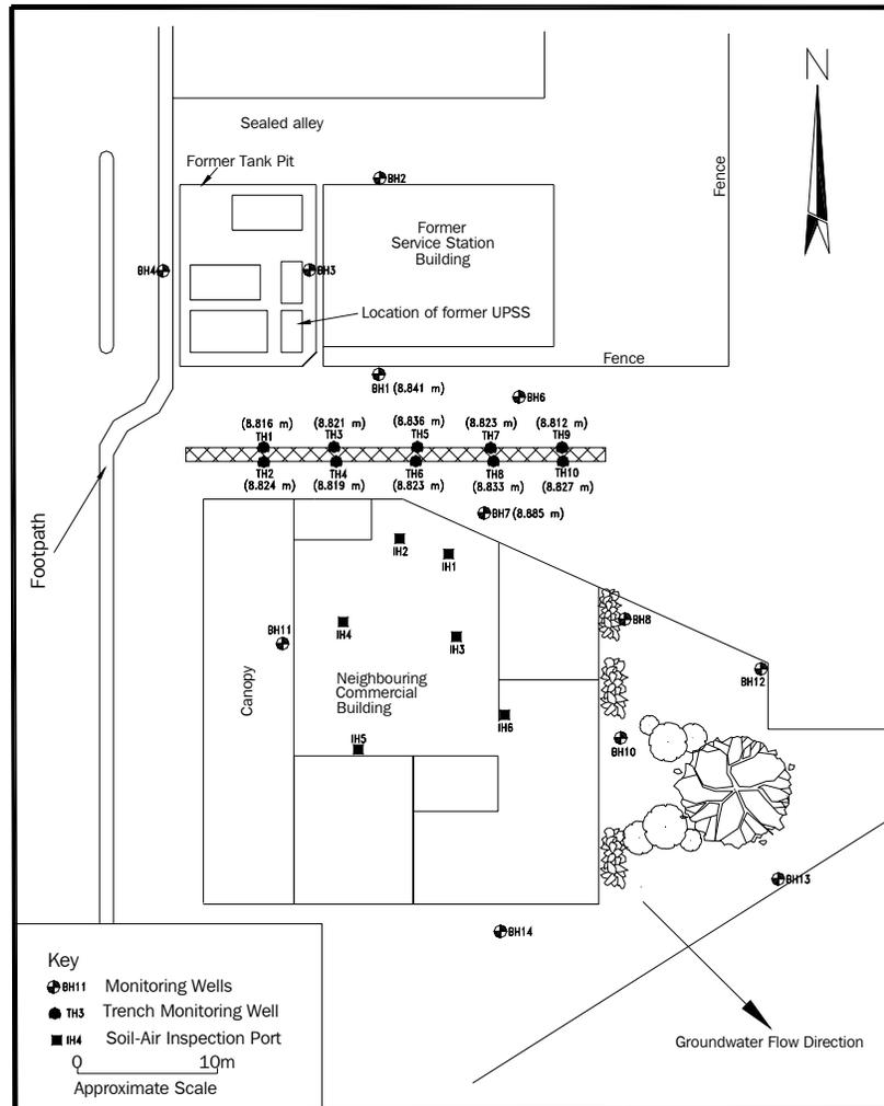
Figure 4: SPH Levels Relative to an Arbitrary Datum (Jan 1998)
