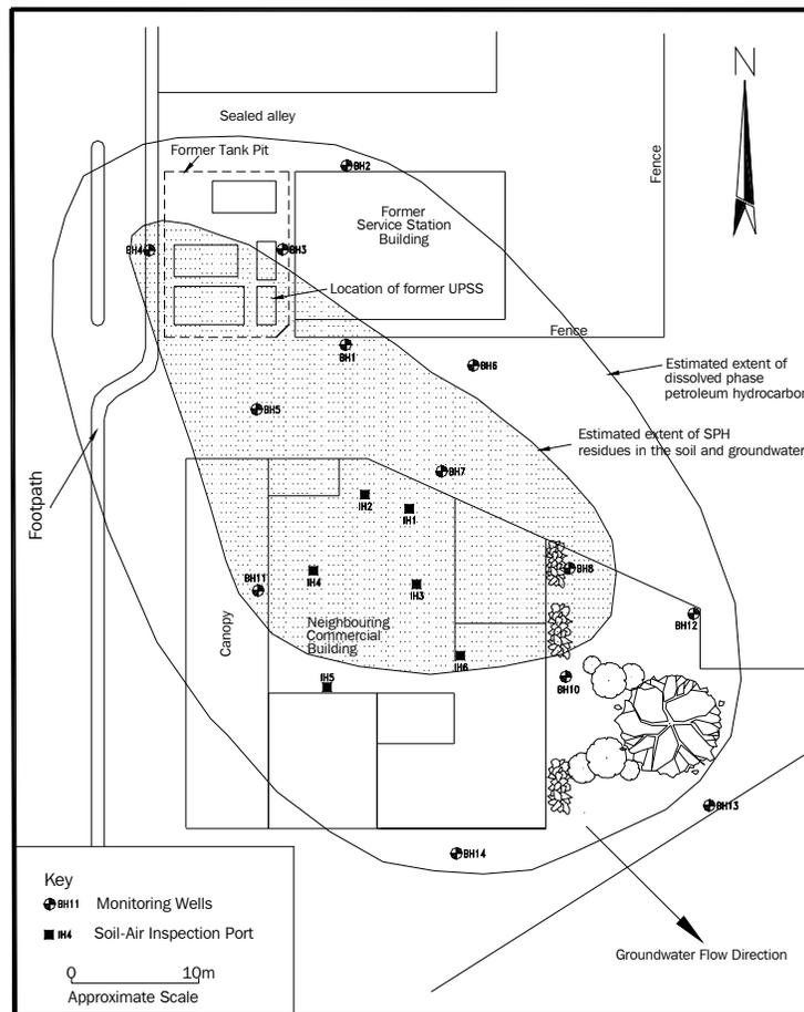
Figure 1: Site Plan and Estimated Extent of SPH Plume (May 1996)
