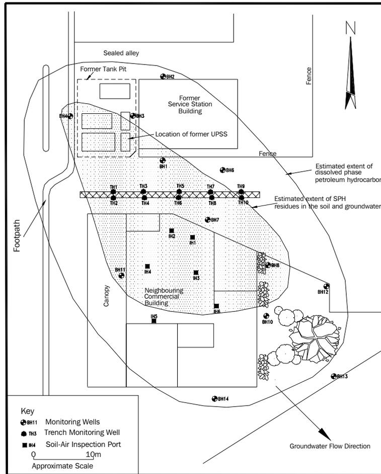
Figure 3: Site Plan showing location of Barrier Trench (Feb 1997)
