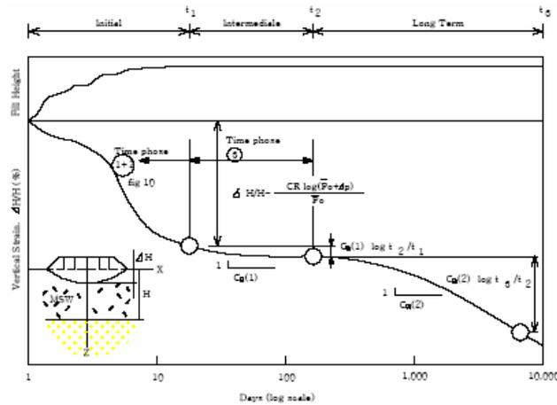
**Figure 1: Idealised settlement model (Pump, 1998 after Bjarngard & Edgers, 1990)**
