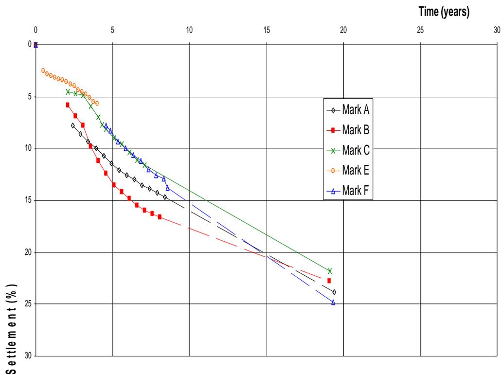
**Figure 2: Measured Greenmount settlement on normal time**
