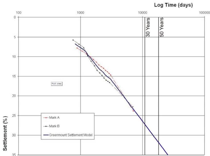
Figure 4: Greenmount Settlement Model (settlement v's log time)
