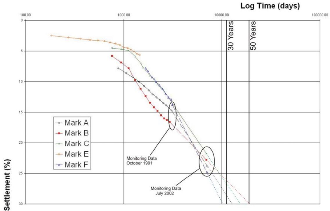
**Figure 3: Greenmount settlement on Log time (Linear extrapolation)**
