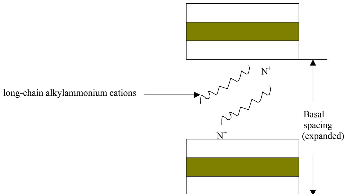
Figure 2. Montmorillonite intercalated with quaternary ammonium cations. Intercalation causes a large expansion of the interlayer space, and increases the capacity of the clay to take up organic pollutants.
