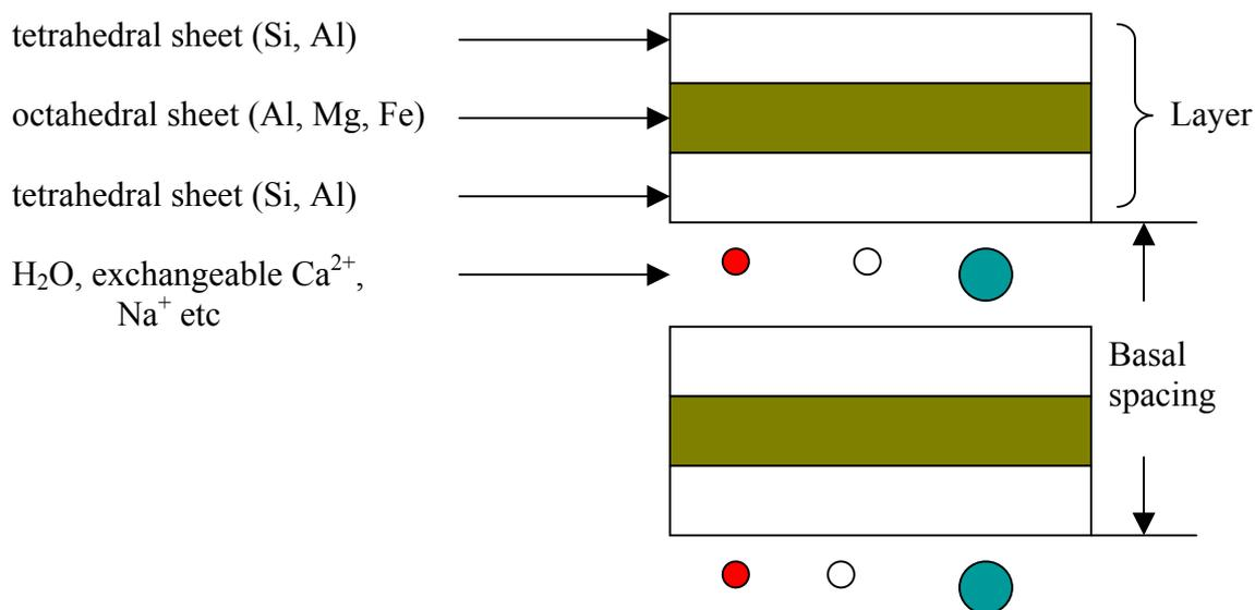
Figure 1. Schematic structure of a montmorillonite clay, showing the arrangement of octahedral and tetrahedral sheets in individual layers. Inorganic cations and water occupy the interlayer space, giving a characteristic basal spacing.
